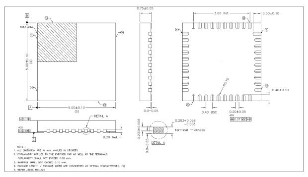
Figure 38: Package Dimensions QFN
