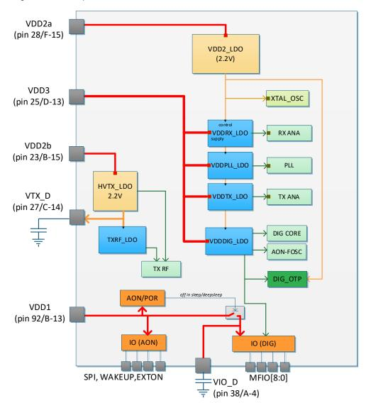
Figure 31: Internal power distribution
