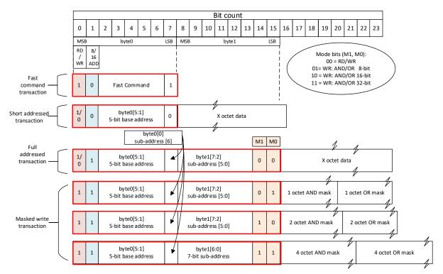
Figure 16: SPI Command Formatting
