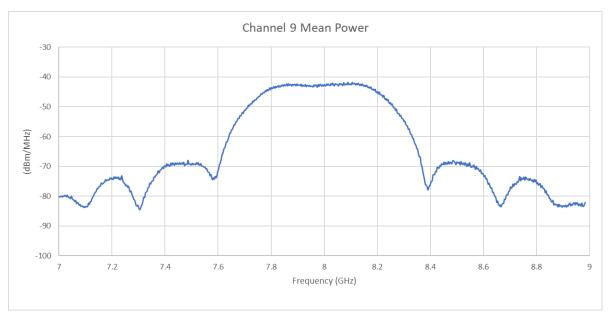
Figure 5: Typical Transmit Spectrum Channel 9
