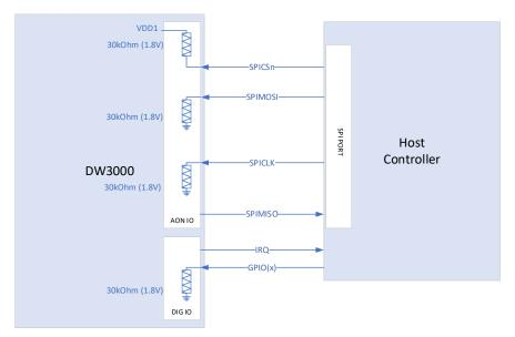
Figure 17: SPI and GPIO pull up/down
