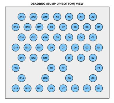
Figure 3: The WLCSP pin assignments
