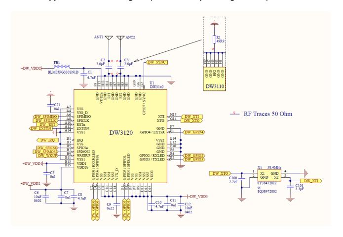
Figure 32: DW3000 WLCSP Application Circuit
