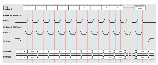
Figure 15: DW3000 SPIPHA=1 Transfer Protocol
