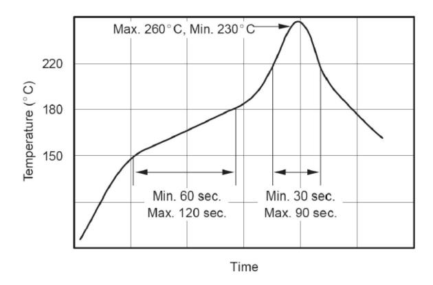
Figure 36 Reflow Profile of the WLCSP package
