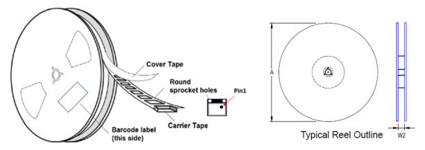
Pin1 Orientation In Carrier Tape
