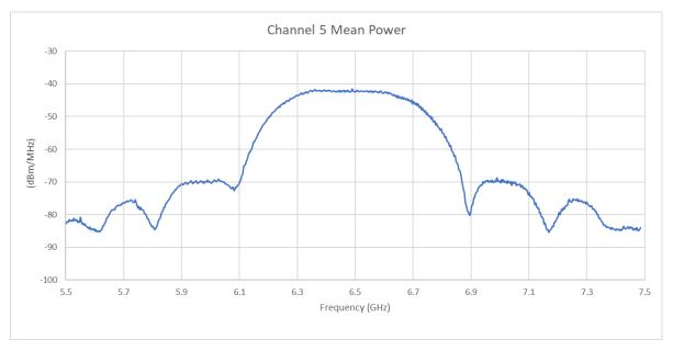
Figure 4: Typical Transmit Spectrum Channel 5
