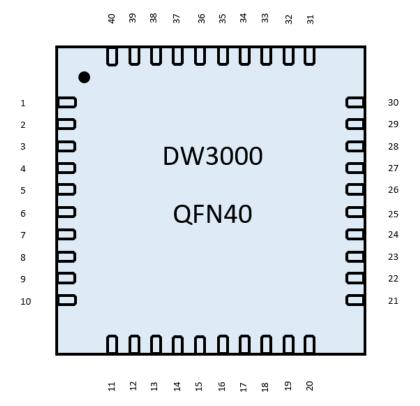
Figure 2: The QFN Top view pin assignments
