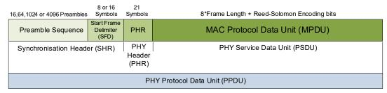
Figure 12: IEEE802.15.4-2011 PPDU Structure
