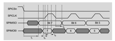
Figure 13: SPI Timing Diagram
