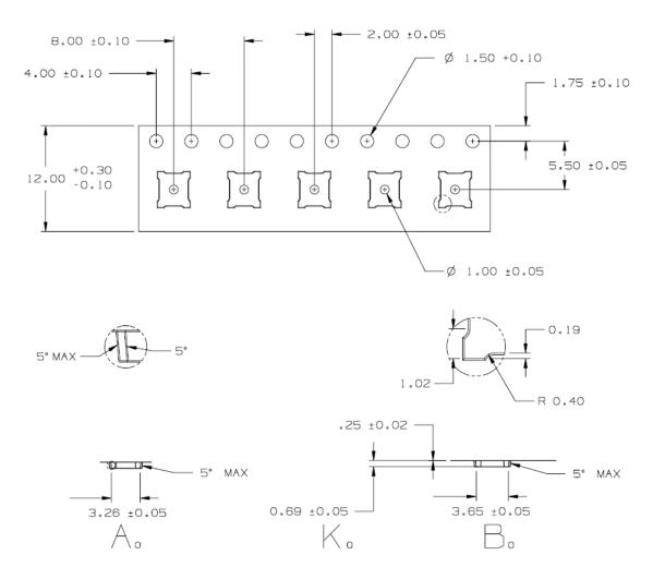
Figure 41 WLCSP Tape Orientation and Dimensions
