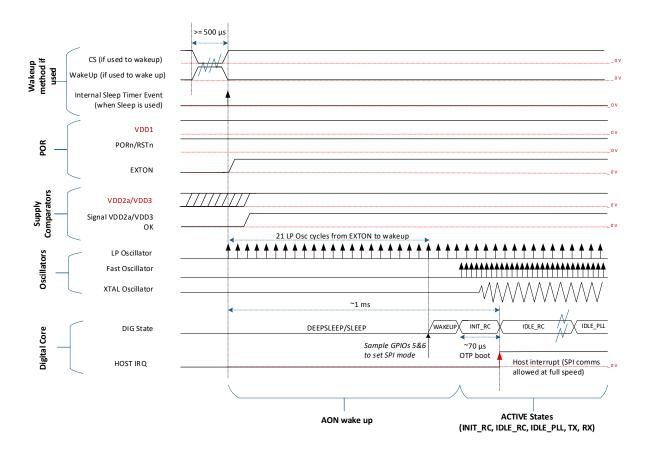
Figure 22 Timing diagram for warm start
