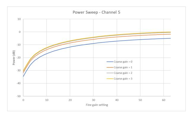
Figure 6 Tx power coarse and fine gain settings - Channel 5
