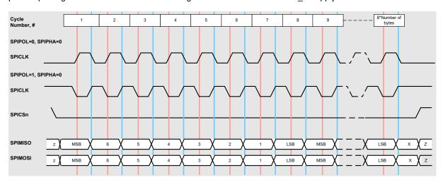
Figure 14: DW3000 SPIPHA=0 Transfer Protocol
