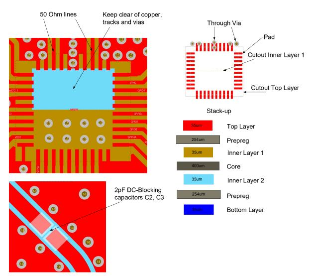
Figure 35 Recommended QFN Stack-up
