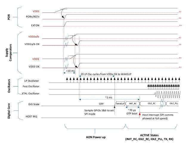
Figure 21: Timing diagram for cold start POR
