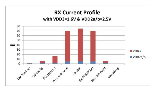
Figure 29: Current consumption during RX for high efficiency powering modes
