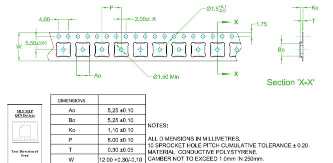
**Figure 39 QFN Tape Orientation and Dimensions**
