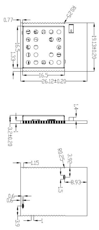
Figure 5: Module Package Size (units: mm)
