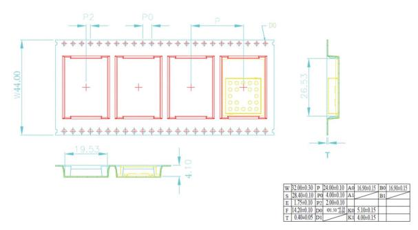
Figure 9: Module and tape dimensions
