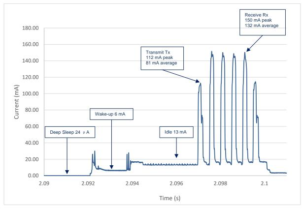
Figure 2: Power consumption running PANS R2 tag application Single Sided Two-Way Ranging scheme
