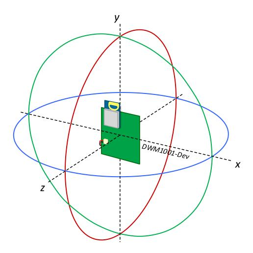
Figure 3. Antenna Radiation Pattern Planes
