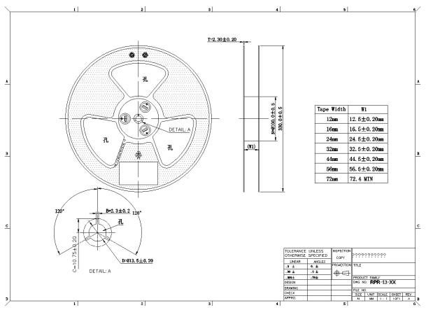
Figure 8: DWM1001 Tape and Reel Dimensions
