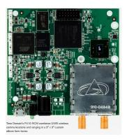
Figure 5.2: Time Domain real time location technology (P410) (from the Time Domain website : www.timedomain.com/).
