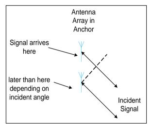
Figure 7: PDoA antenna array
