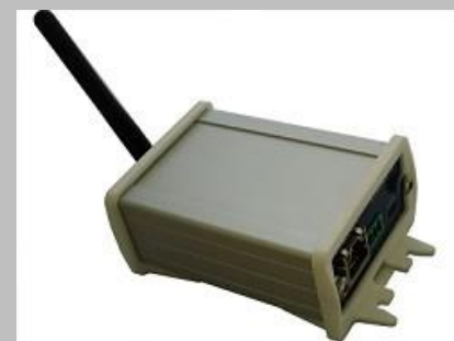
87x64x40mm anchor unit from REK1101
