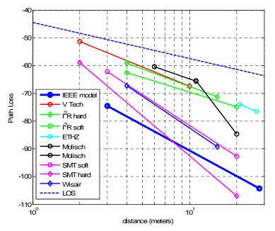
Figure 1. Different path loss models for UWB channels
